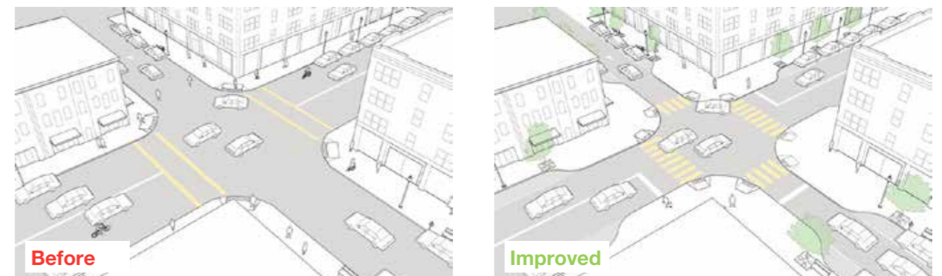
Figure CP.9. Pedestrian areas will be designed as shared spaces with pavement crossovers at junctions.
