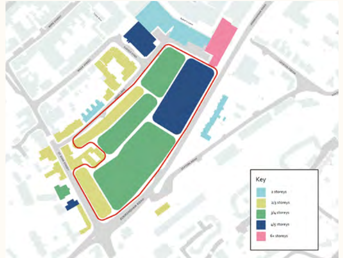
Suggested height plan: higher densities are permissible closer to the former Debenhams building on the northeast of the site.
