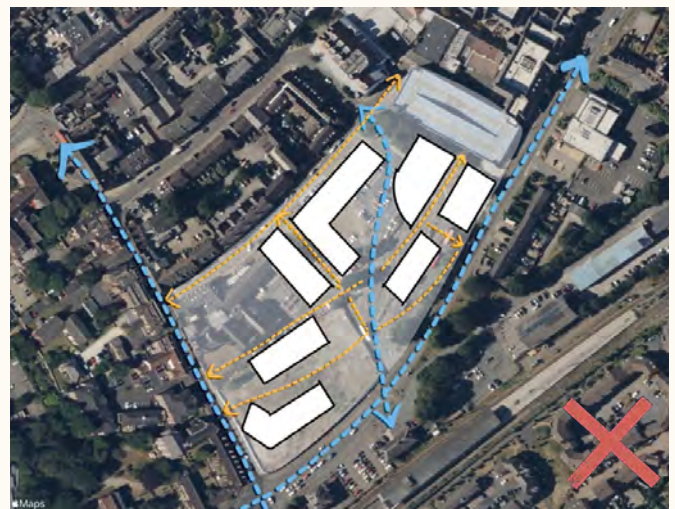
Indicative example: here the blocks do not define routes and routes do not define the blocks, creating illegible space.
