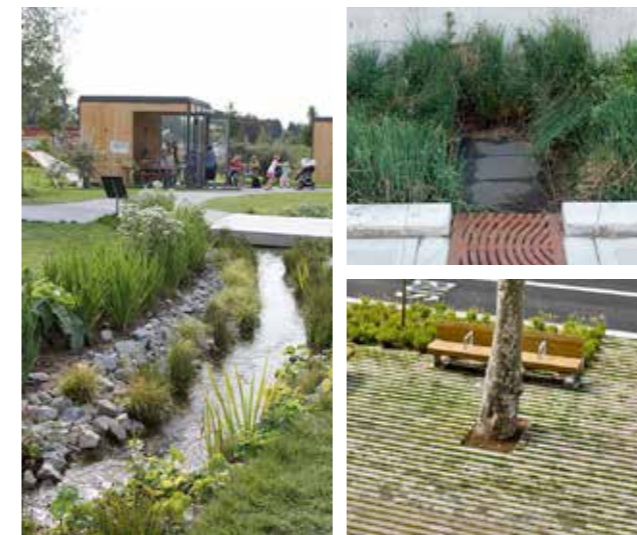
Figure CC.22. Example of surface run-off treatment
