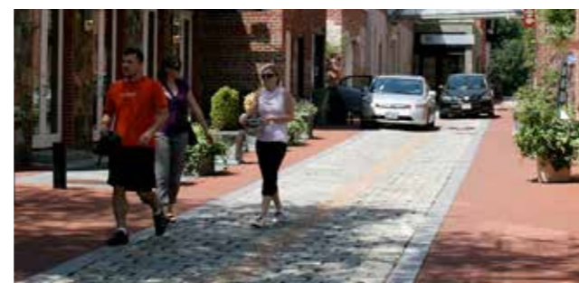
Figure SU.7. Footways should be delineated by low kerbs at shared space.
