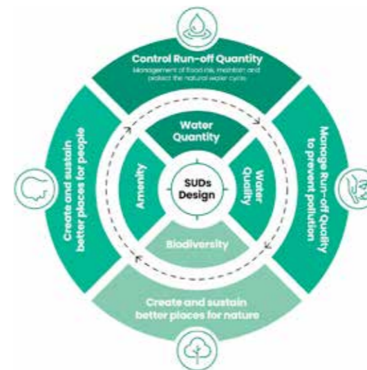
Figure RA.4. Four Pillars of SuDS Design. ©The SuDS Manual C753, Ciria
