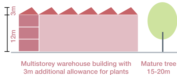
Figure EA.26. Typical Section of employment building
