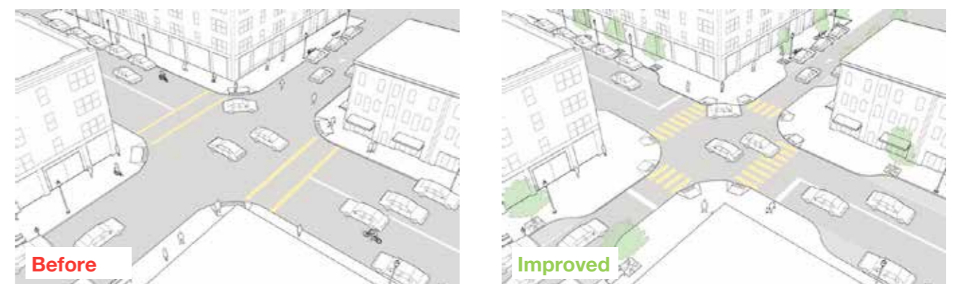
Figure CP.9. Pedestrian areas will be designed as shared spaces with pavement crossovers at junctions.
