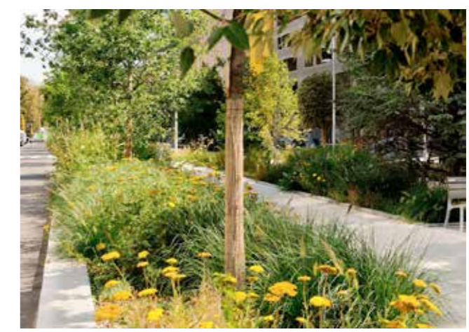
Figure SU.57. Rain gardens along streets to help with rain water management
