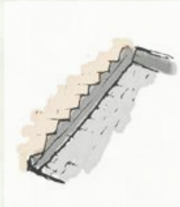
(Figure 10: Stepped Lead Flashing)
