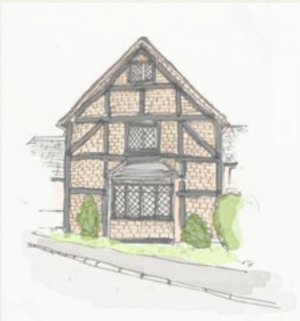
(Figure 9: Timber Frame Brick Infill Gable)
