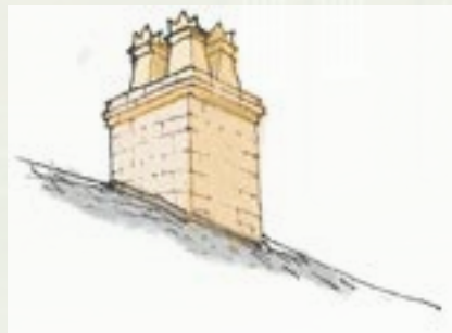
(Figure 15: crenelated chimney pot)
